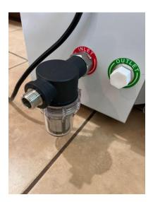
• Unscrew the clear, plastic cartridge filter housing in the back of the chiller by turning it clockwise. You can do this with your hand, or with the plastic white wrench found in the spare parts bag. You'll then place the white cartridge filter into the housing, and screw the housing back into place.
