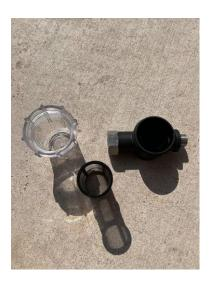
Check the cartridge filter regularly, and replace it when the color begins to turn light brown,
